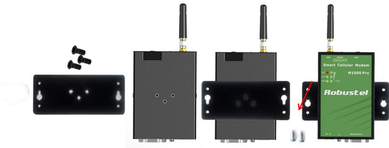
2. Mount the Gateway on a DIN rail with 3 pcs of M3 screws, and then hang the DIN-Rail on the holder. You need to choose a standard holder.
