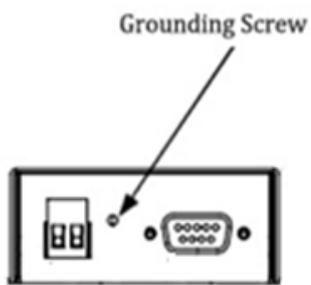
Grounding and wire router helps limit the effects of noise due to electromagnetic interference (EMI). Run the ground connection from the ground by screwing to the grounding surface before connecting devices.
