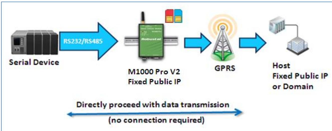
1. If your cellular ISP offers a fixed public IP address after you connect to the cellular network, you can access the gateway from a host PC that has a fixed public IP bidirectional.
