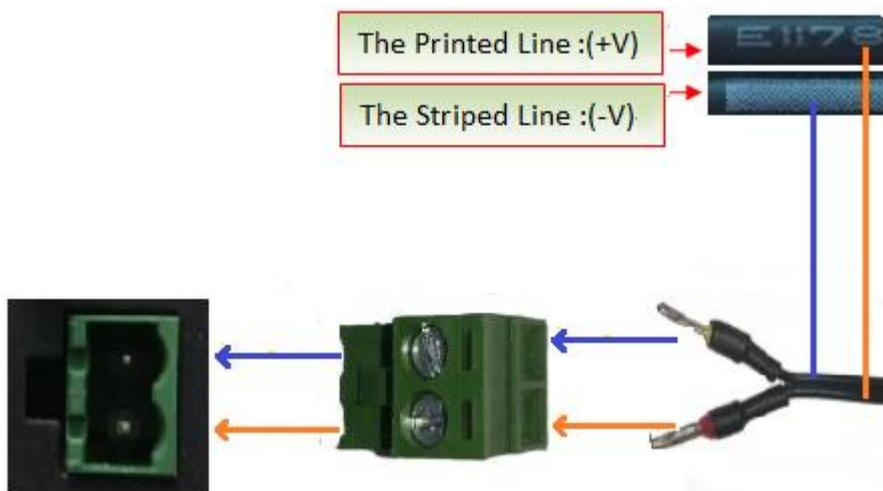
The power supply range is 9 to 36VDC.
